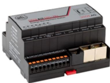
You can now connect up to two M-bus interfaces each with 60 meters to the OPEN 710 or 810 EMS + M-Bus directly and without any level converters.
